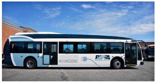
Notes: This electric bus was leased in RIPTA's Zero Emissions Vehicle Program Pilot. The bus has a larger battery system that is designed to be charged slowly overnight when the bus is not in use.
