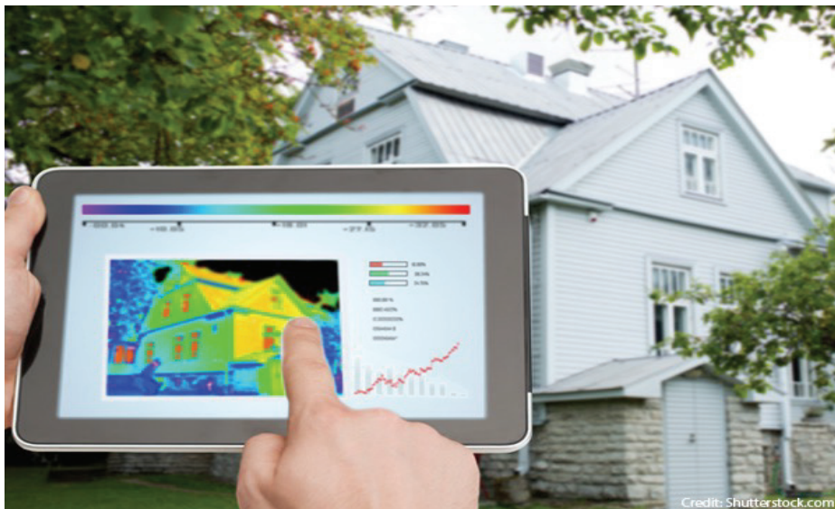
Figure 3: A thermographic representation to detect air leaks and insulation gaps
