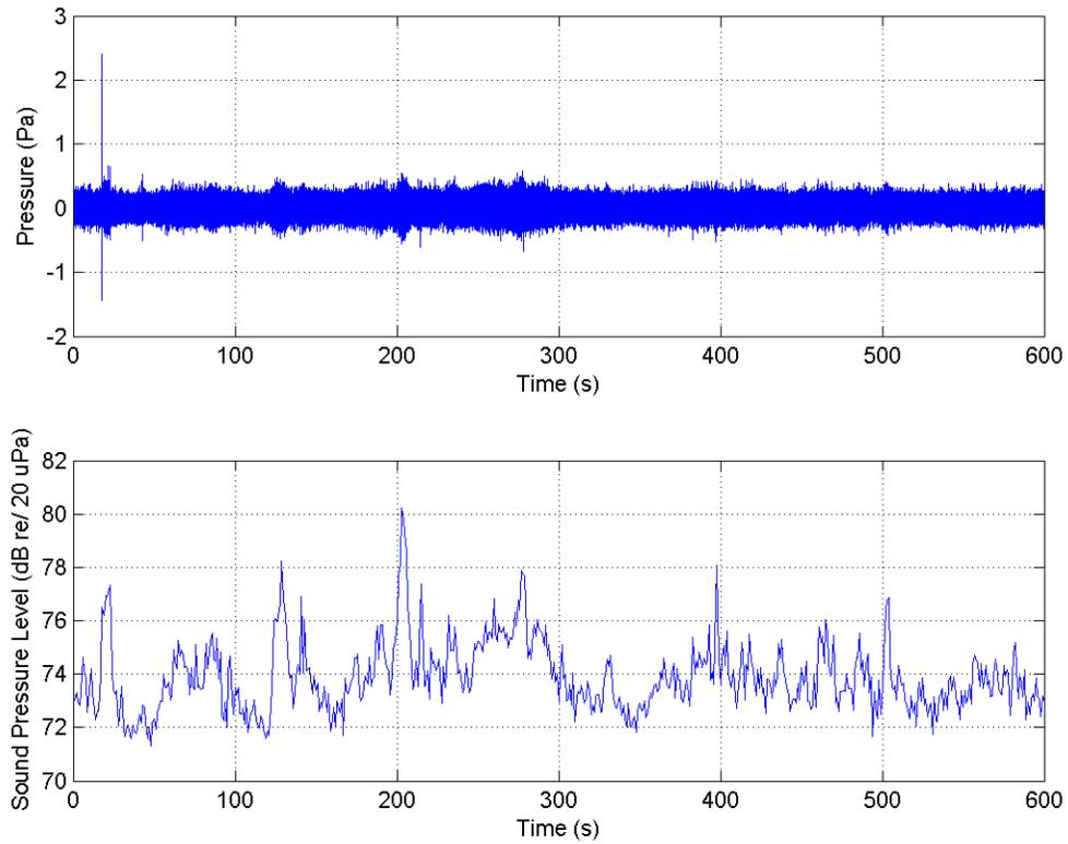
**Figure A.64:** Infrasound Data Recordings at Shalom Housing 05 NOV 2013 at location 41 43 27.12 N, 71 27 59.82 W. (Channel 2 Time Series).
