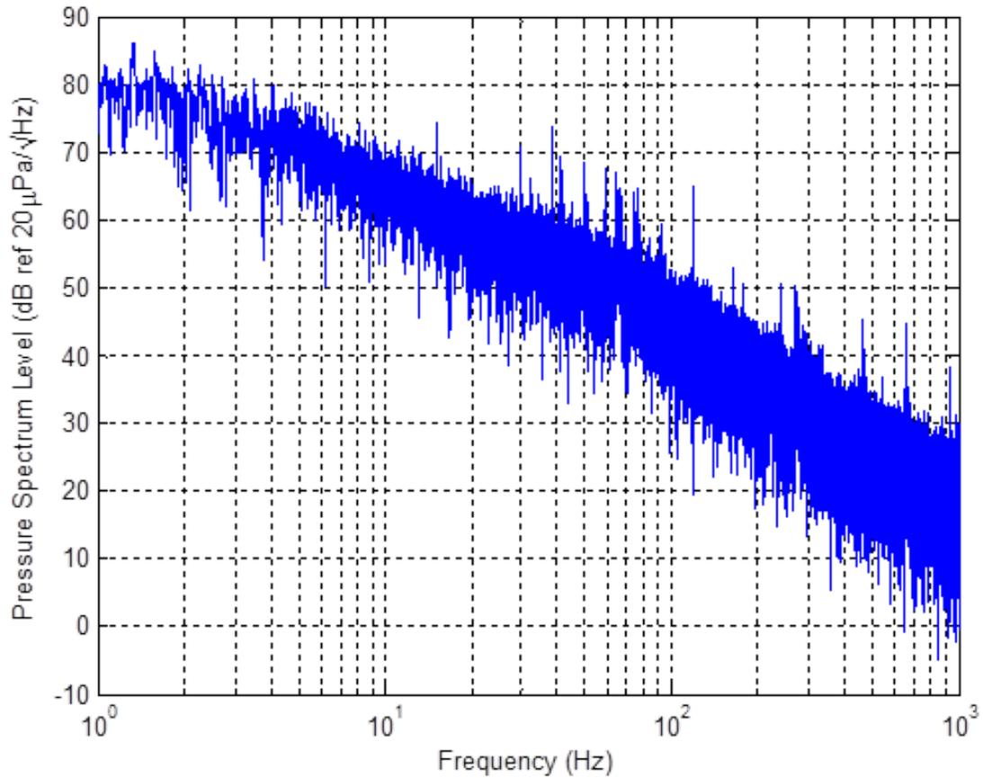
**Figure 4.5:** The voltage time series (converted to pressure time series using each microphone sensitivity) yields the un-weighted Pressure Spectrum Level. This representation shows the distribution of acoustic power as a function of frequency. Most of the acoustic power is concentrated in the low frequency (20-200 Hz) and infrasonic frequency (1-20 Hz) bands.
