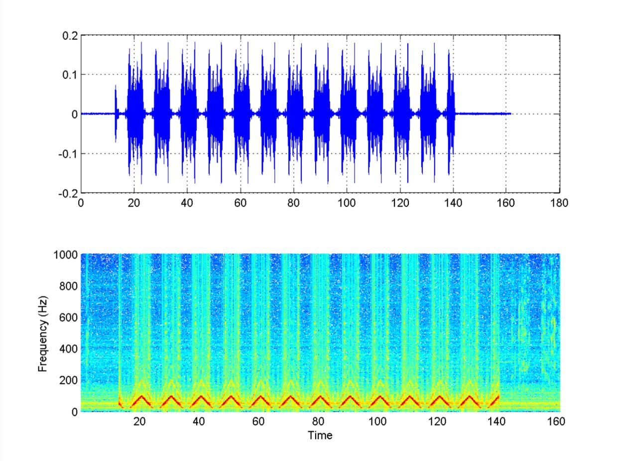
**Figure 2.4:** Voltage Time Series and Spectrogram for TASCAM recording system for LFM calibration signals.
