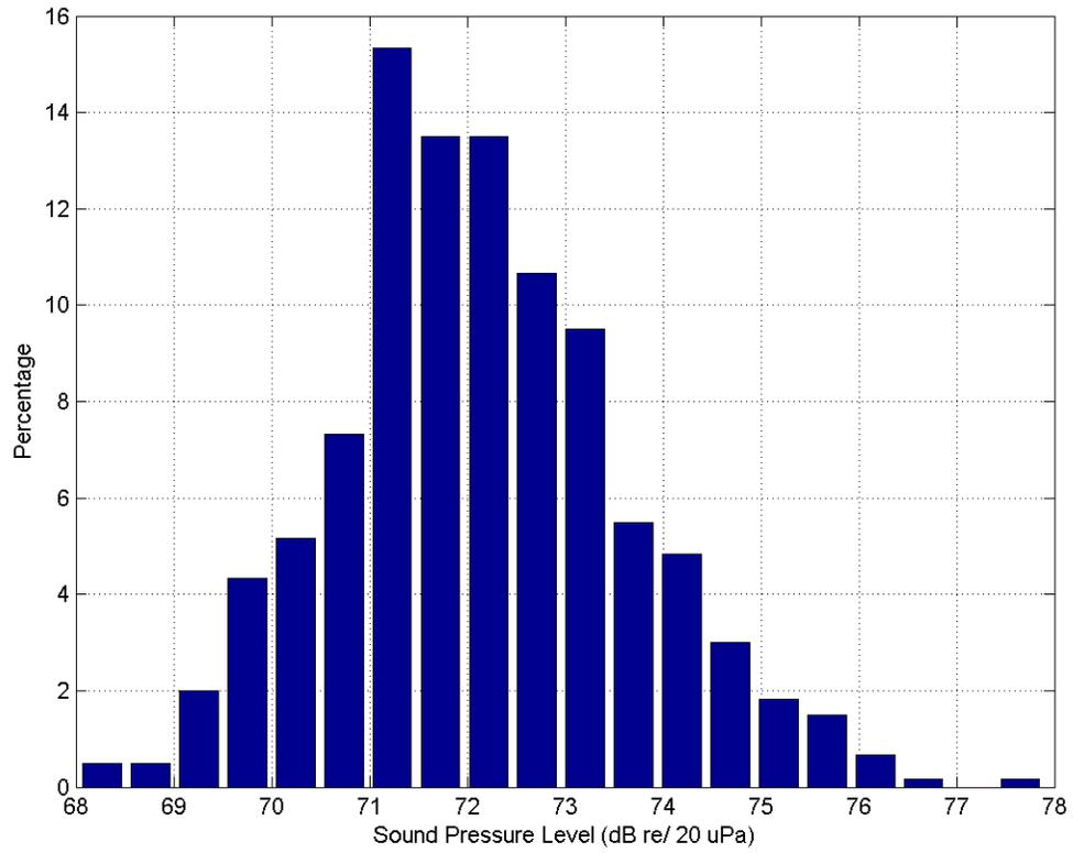
**Figure A.67:** Infrasound Data Recordings at Shalom Housing 05 NOV 2013 at location 41 43 25.86 N, 71 28 01.02 W. (Channel 2 Histogram).
