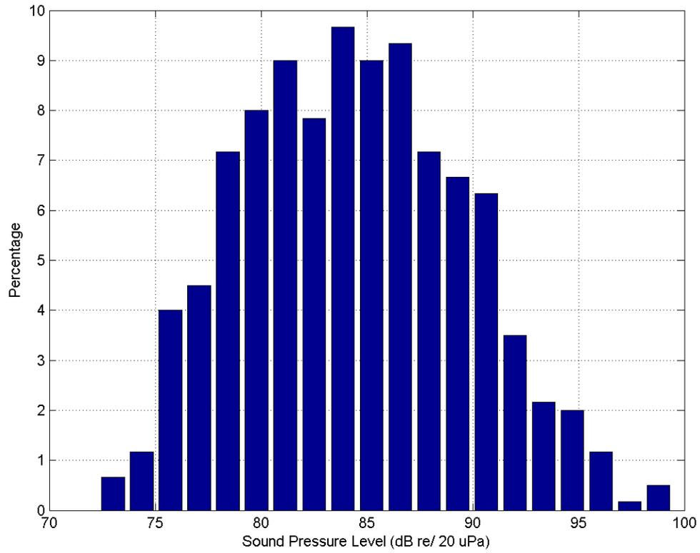
**Figure A.43:** Infrasound Data Recordings at New England Inst. of Technology 27 OCT 2013 at location 41 44 04.01 N, 71 27 00.33 W. (Channel 2 Histogram).
