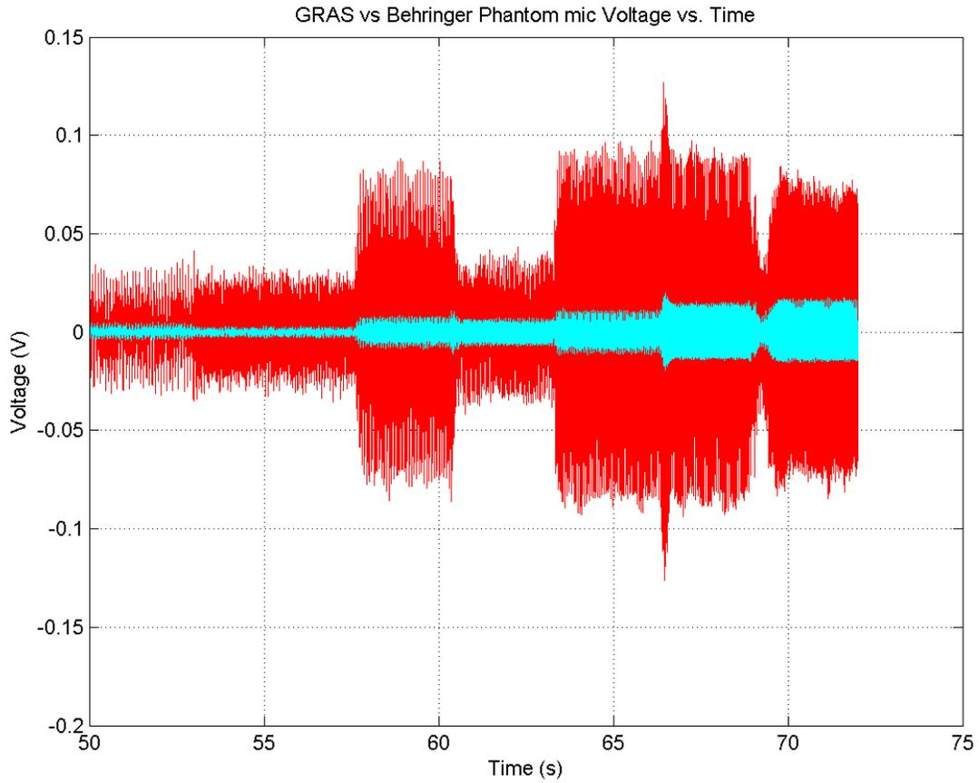
**Figure 2.6:** Comparison of Voltage Time series between Infrasonic system and TASCAM system. The TASCAM and Infrasonic System have different sensitivities (how much voltage is output for the same sound pressure). Because of this the blue signal and red signal have different amplitudes. But the ratio between them is in agreement based on these different sensitivities.
