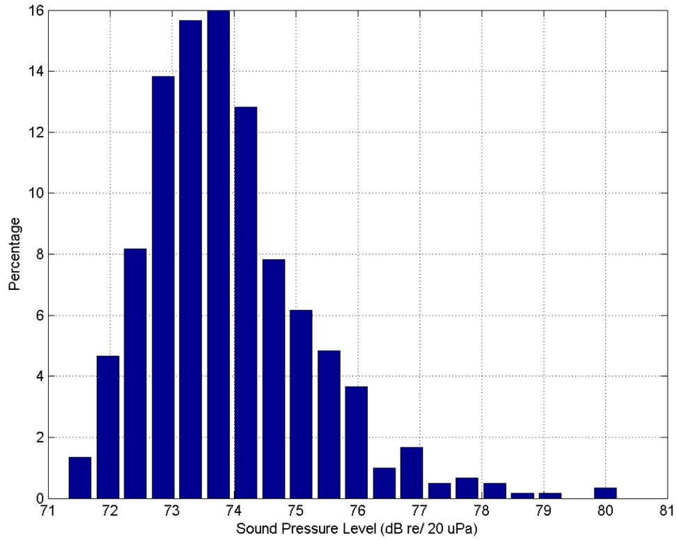
**Figure A.63:** Infrasound Data Recordings at Shalom Housing 05 NOV 2013 at location 41 43 27.12 N, 71 27 59.82 W. (Channel 2 Histogram).
