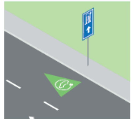
FIGURE 13. WAYFINDING SIGNAGE DIRECTS DRIVERS TO EV CHARGING STATIONS AND CAN INDICATE WHAT TYPE OF EVSE IS AVAILABLE.
